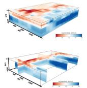
3-D Omo resistivity model. The survey provided an accurate estimation of the sedimentary basin geometry
